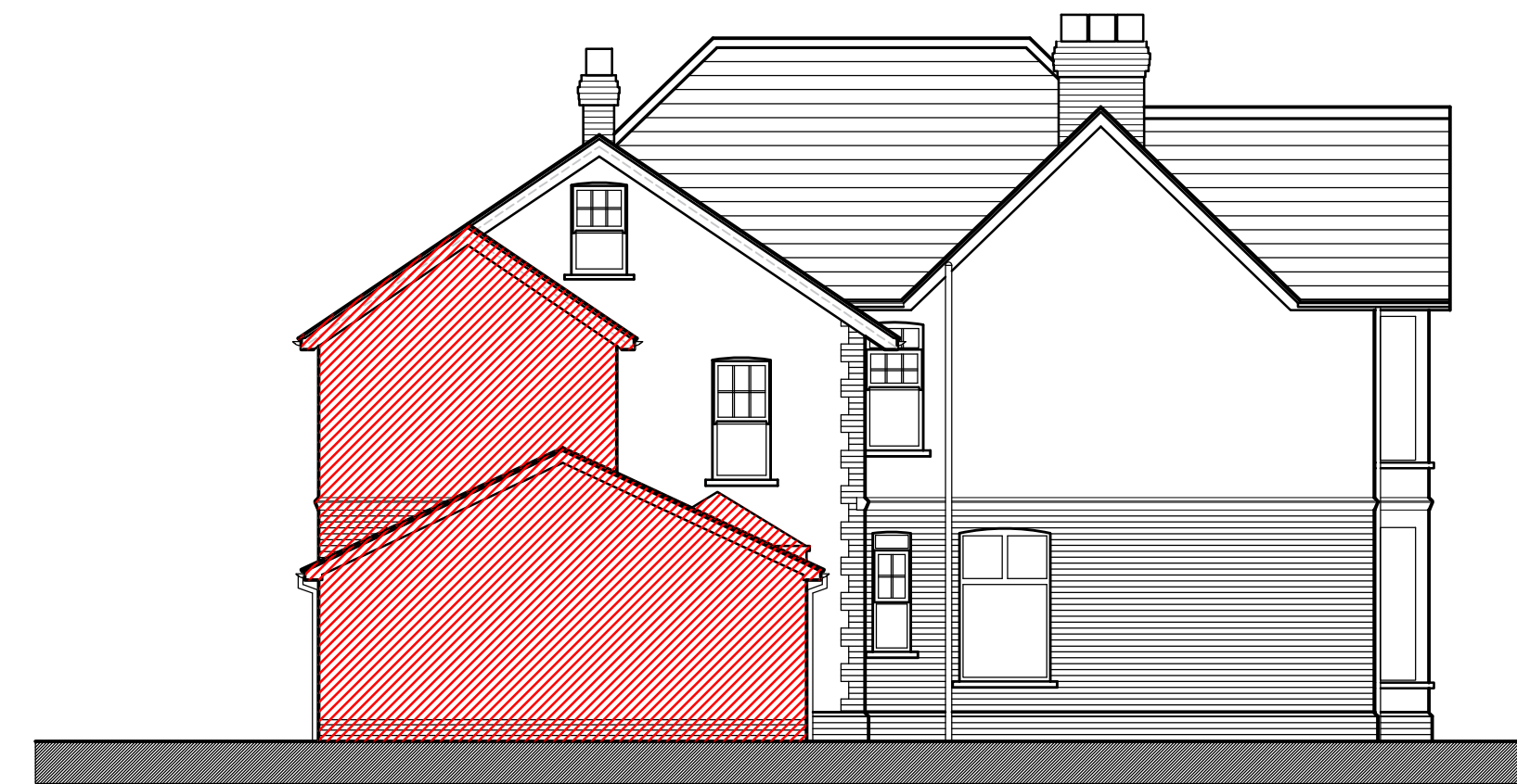
Existing Elevation to No 3 Westbourne Crescent Showing Demolitions
